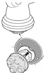
Choose the desired accessory for the massage, mount it onto the hexagonal base making sure that the apparatus is both switched off and unplugged.
