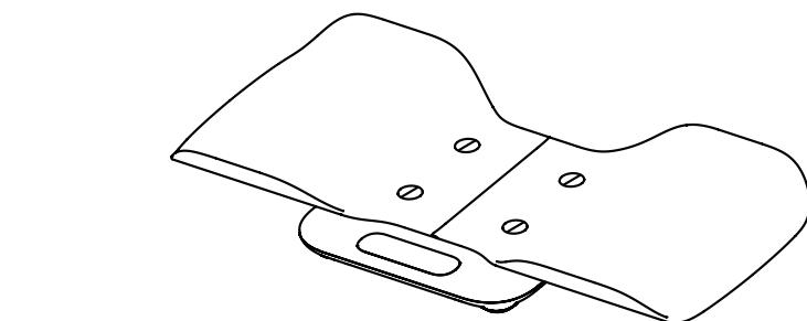
Loosen the screws with the coin-shaped screwdriver
