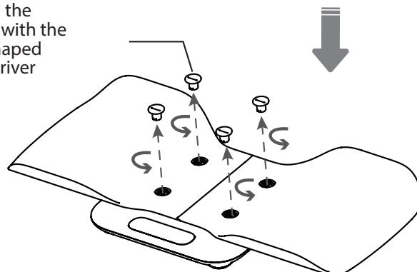
Tighten the screws with the coin-shaped screwdriver
